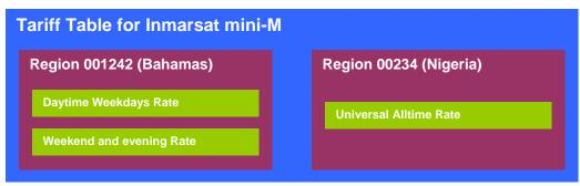
A **Tariff Table** is a collection of Regions and Rates which together are used for calculating the call cost for each phone call via the Tel-Log unit. One example of a Tariff Table would be "**Inmarsat mini-M**". This table would then hold one Region for each distinguishable dial string.
